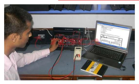
46905 is a platform where Students can understand the various thyristor firing technique by using IC 555 and UJT. This is very useful for understanding of pulse generation. 2703 is provided with in built power supplies, sockets for making interconnection in the circuit and exhaustive learning material.
