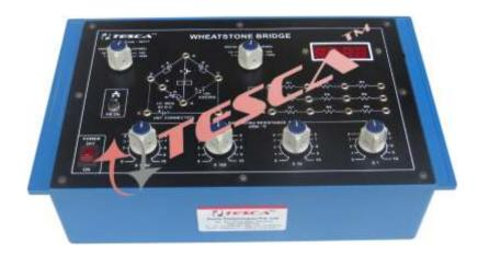
Experimental Training Board has been designed specifically for the study of Wheatstone Bridge. Using this bridge the value of unknown resistor can be found. The board is absolutely self contained and requires no other apparatus.
