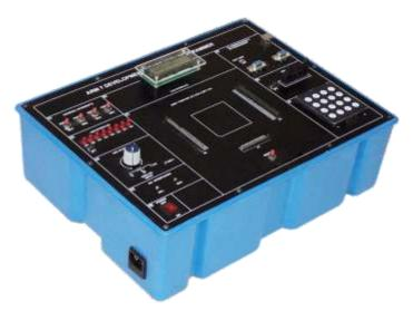
ARM 7 Development Board 43558 is a 32-bit development platform and serves as a means for code development. This trainer is designed for students to explore ARM architecture and on board supporting peripherals which provide an ideal platform for extensive embedded development. This trainer provides both the serial and USB connections which can be used to download and run a code on any standard IDE. This trainer allows users to evaluate, prototype and create application specific designs.
