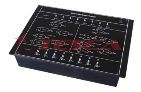
38716 Experimentation with Universal Gates-Nand and Nor laboratories. It is useful for understanding of the basic concepts and functioning of universal gates as well as their use as other logic gates.
