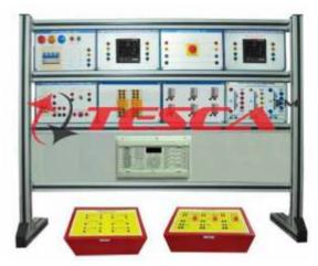
Order Code - 46641 Distance Protection Relay Trainer Is a rouged training system for the Electrical laboratories mounted on Aluminum profile rack with sturdy table top flat panel. Each panel has ABS molded plastic sturdy enclosure with 4mm shrouded connectors showing circuit diagram & its connection tag numbers for easy understanding and connections. The product helps you to get fully acquainted with the basic concepts and functioning of a Distance Protection Relay Trainer
