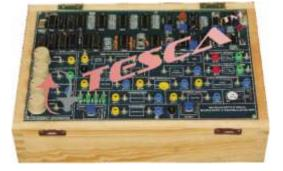
**Order Code-40615** is a Digital Communication Trainer System to under stand various digital Modulation and Demodulation Techniques. Various functional block diagrams are provided on-board for Teaching/Training. This Kits provides with various Test Points to visualize the signals on Oscilloscopes.
