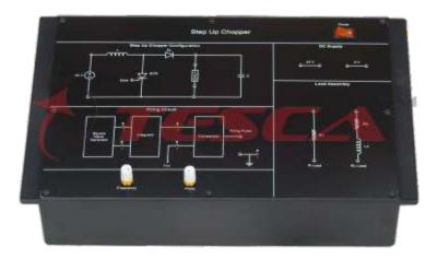
46914 is a learning platform which is very useful for Students to understand the concept of thyristor firing method & working of DC to DC conversion on various load configurations. Platform is provided with inbuilt DC power supply & exhaustive learning material.
