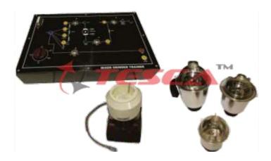
10955 Mixer Grinder Trainer is an ideal training equipment to teach the operation of Mixer Grinder. The complete Block of Mixer Grinder is printed on single PCB for easy understanding of function of different blocks. Test points allow the analysis and monitoring of the signals in different sections. By using the fault simulation method, it is possible to introduce the most common breakdown and their rectification.
