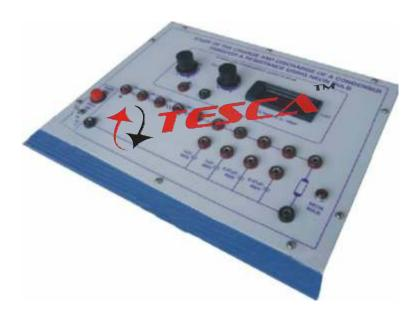
Experimental Training Board has been designed specifically to study the Charge and Discharge of a condenser through a resistance using neon bulb.
