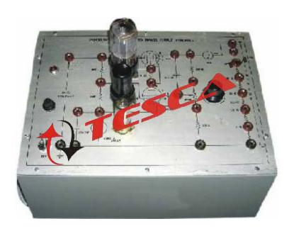
Experimental Training Board has been designed specifically for the study of Electronically Regulated Power Supply. By this Training Board one can study the effect at output by variation of load and line voltage at input.
