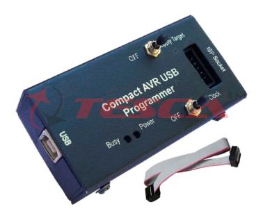
Compact AVR USB Programmer 43561A is designed for ATMEL ATmega, Tiny & AT90 series Microcontroller. It is a full featured USB in-circuit programmer for Atmel AVR microcontrollers. This USB programmer will easily connect with PC and laptops. It comes with Programmer Software which allows user to perform various commands like Read chip signature, Erase, Read/Write, Verify and Fuses/Lock bits setting.
