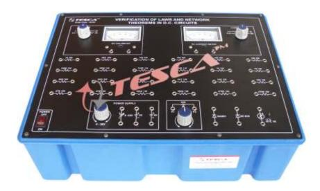
Experimental Training Board has been designed specifically for the study & verification of the laws and network theorems in D.C. circuits. The board is absolutely self contained and requires no other apparatus.
