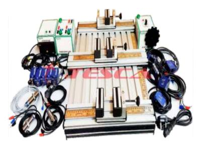
**52085.1** is a Digital Sensor Workstation consisting of instrument panel and working table suitable for students to learn and perform various experiments related digital sensors. Single phase 230V, 50 Hz input supply sockets are provided on the unit.
